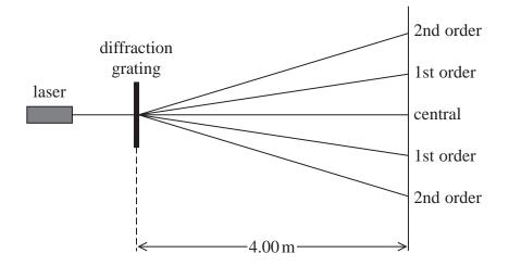
The diffraction grating has  $4.00 \times 10^2$  lines per millimetre.
