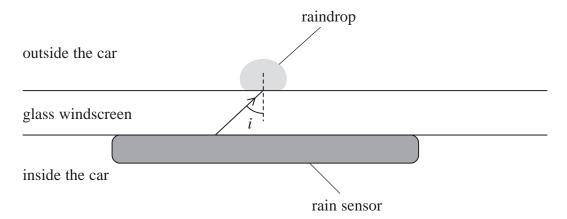
The angle of incidence i is  $45^{\circ}$ .
