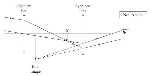
The objective lens produces an inverted image at point X. The image at point X is the object for the eyepiece lens. The eyepiece lens produces a magnified image.
