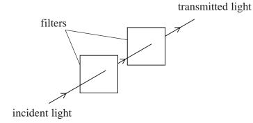
One filter is rotated so that the planes of polarisation of the two filters are perpendicular.
